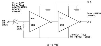
Simple driver using inexpensive standard logic ICs provides fast switching using minimum DC current while translating from standard positive voltage TTL or CMOS logic to negative voltage GaAs IC logic.
